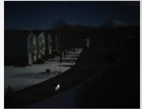
Figure 5: Another image generated by the pinhole camera. But this image was captured with 15 seconds exposure time. Longer exposure time (Figure 3) works well for capturing images in low lighting conditions.
