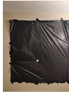
Figure 4: My apartment window was blocked using an opaque sheet to construct the camera. A pinhole was made in the sheet so that the light generates an image on the opposite wall (Figure 3)
